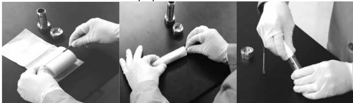
Accelerated Solvent Extraction (ASE) of Polychlorinated Biphenyls from Polyurethane Foam Adsorbent Cartridges (Dionex, application note 333)
