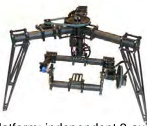
Platform: independent 3-axis stabilization
